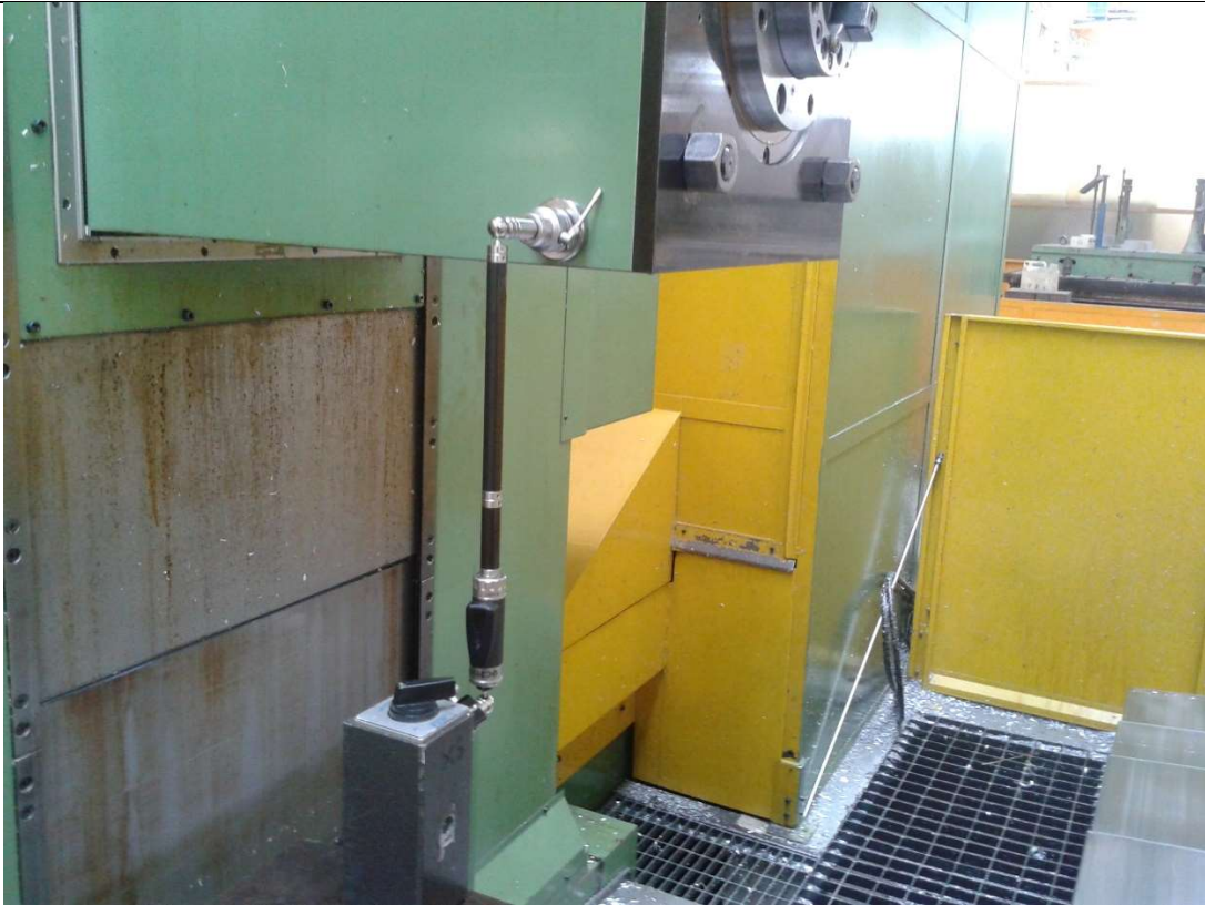
Figure 23 – Milling and boring machine – Measurement in the YZ plane
